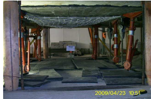
Photo 2: Prior to testing. The 1.5m x 1.5m net installed with a hanging wall to net spacing of 55mm.
