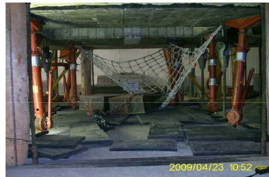
Photo 4: West to east view of the net after the 1m drop test. The net failed on the re-spliced corner.
